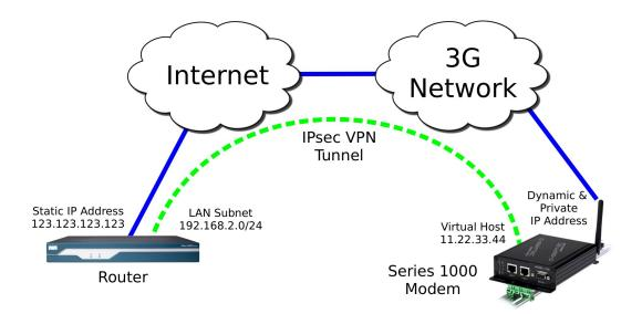
Figure 254: IPsec configuration example network
