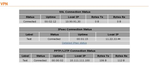
Figure 288: The VPN status page showing 3 active VPN connections
