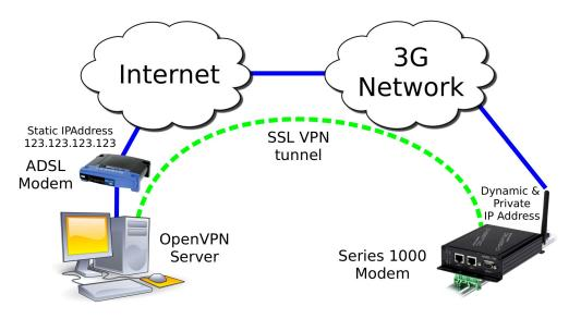
Figure 278: SSL based VPN example network
