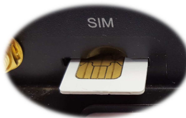
Figure 5: Inserting the SIM card.
