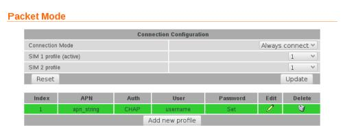
Figure 25: Completed wireless configuration.
