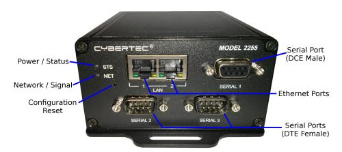
Figure 3: Model 2255 front panel.
