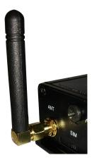
Figure 14: Antenna connected to SMA connector.
