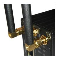
Figure 6: Antenna connected to SMA connector.
