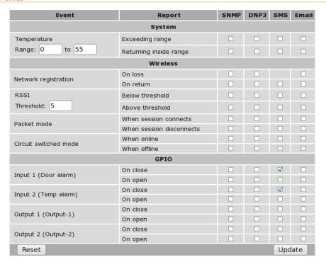
Figure 63: The GPIO SMS event configuration example.
