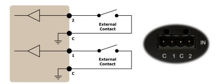
Figure 9: Digital Input circuit and connector.
