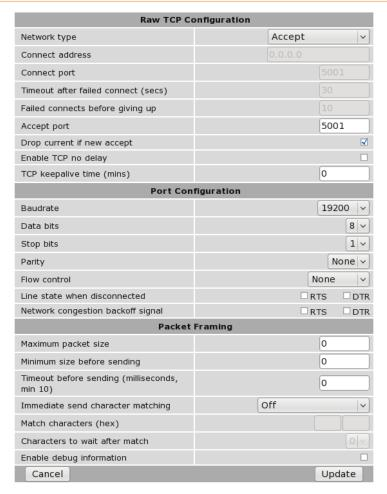
Figure 242: Raw TCP Client/Server configuration
