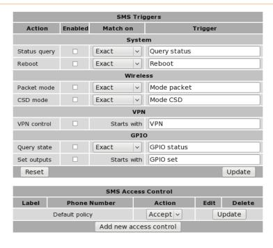
Figure 97: SMS Triggers configuration page for the Model 2220.
