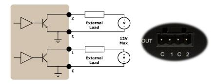
Figure 10: Digital Output circuit connector.
