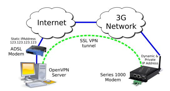
Figure 218: SSL based VPN example network
