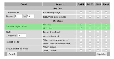
Figure 270: Enabling SNMP traps for the Network Registration events.
