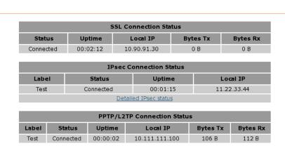
Figure 228: The VPN status page showing 3 active VPN connections
