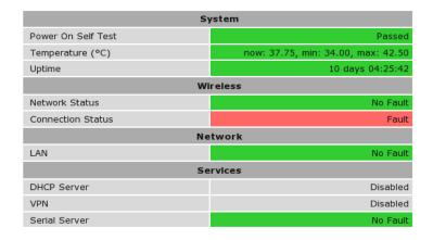
Figure 42: Alarms status page showing Wireless connection status fault.
