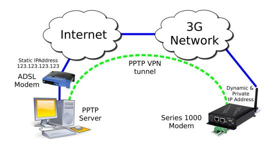
Figure 224: PPTP based VPN example network
