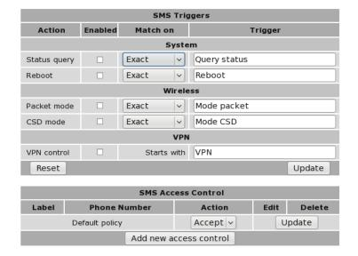
Figure 96: SMS Triggers configuration page for the Model 2100.
