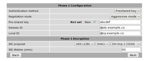
Figure 208: IPsec phase 1 configuration example.
