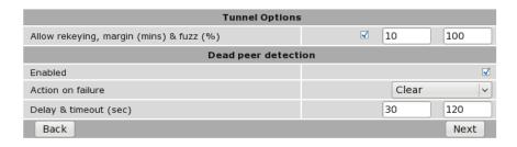
Figure 210: IPsec tunnel options and Dead Peer Detection configuration example.
