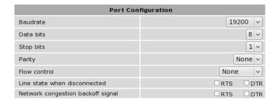
Figure 239: Common port configuration parameters
