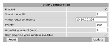
Figure 130: VRRP configuration for Router B.
