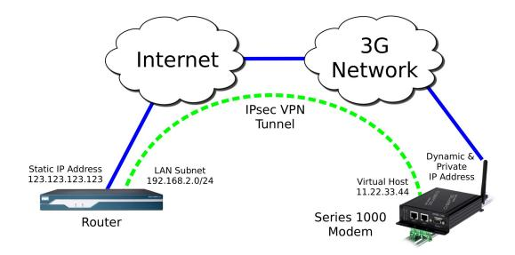
Figure 205: IPsec configuration example network
