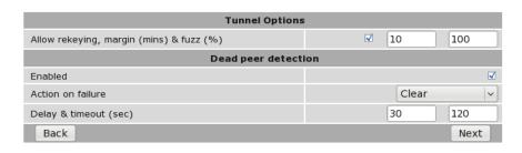
Figure 203: IPsec Tunnel options and Dead Peer Detection configuration.
