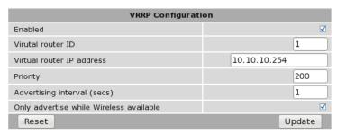
Figure 129: VRRP configuration for Router A
