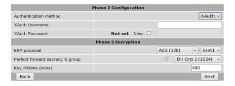
Figure 202: IPsec Phase 2 configuration with Xauth enabled.
