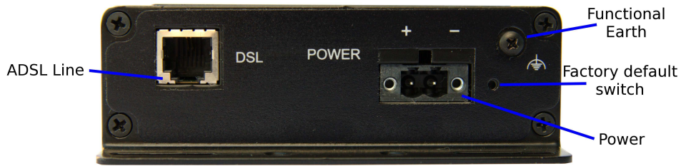
Figure 2: Model 5100 rear panel.
