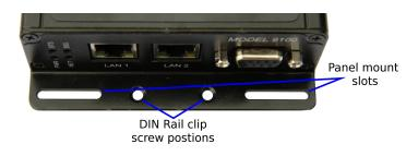
Figure 16: Mounting flange.
