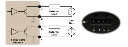
Figure 10: Digital Output circuit connector.
