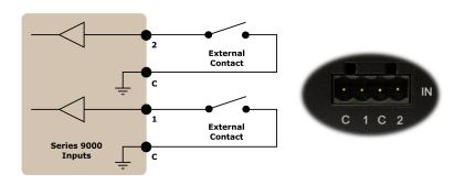
Figure 9: Digital Input circuit and connector.
