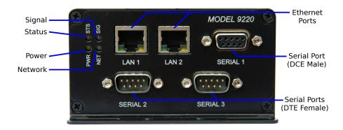
Figure 3: Model 9220 front panel.
