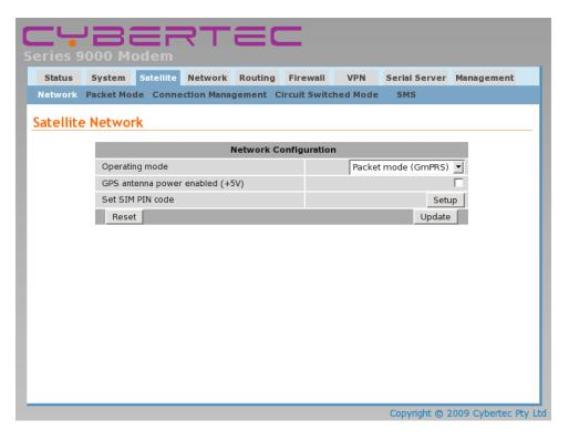
Figure 26: Satellite Network configuration.
