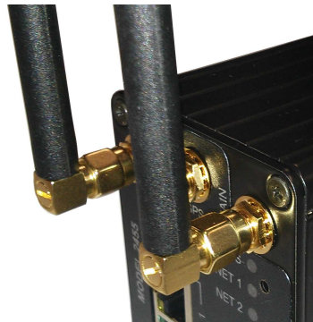
Figure 6: Antenna connected to SMA connector.
