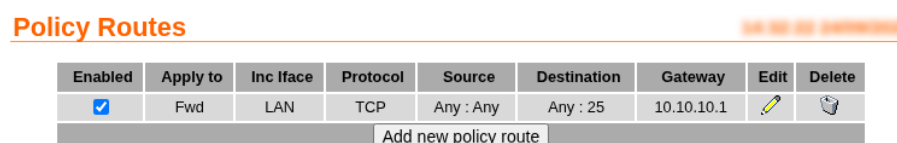
Fig. 9.28: Policy route table with route two removed
